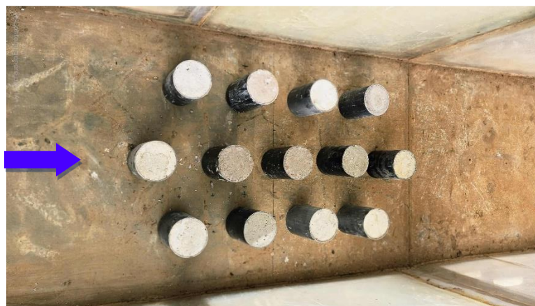
Figure 4. Photograph illustrating the spatial configuration and precise positioning of the cylindrical obstacles within the experimental channel.
