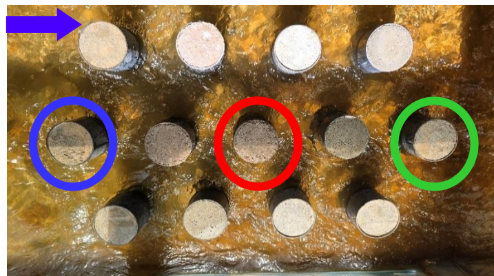
Figure 5. Photograph showing the three measurement locations along the obstacle configuration: upstream (blue), central (red), and downstream (green).
