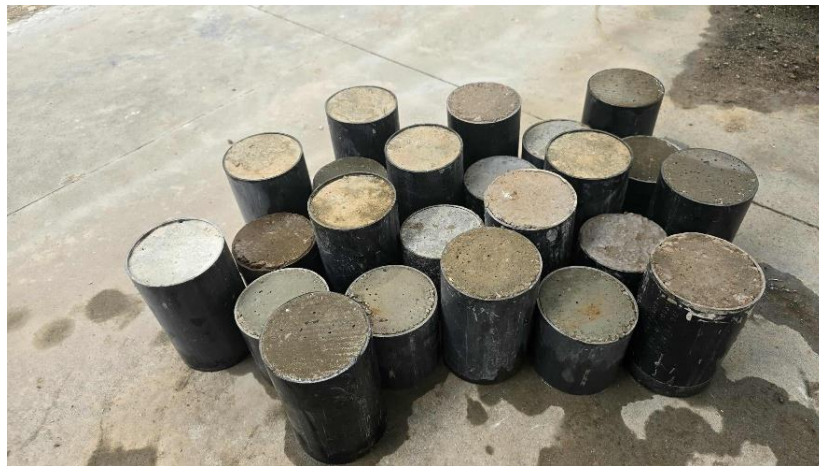
Figure 2. Cylindrical concrete obstacles after fabrication using PVC molds.
