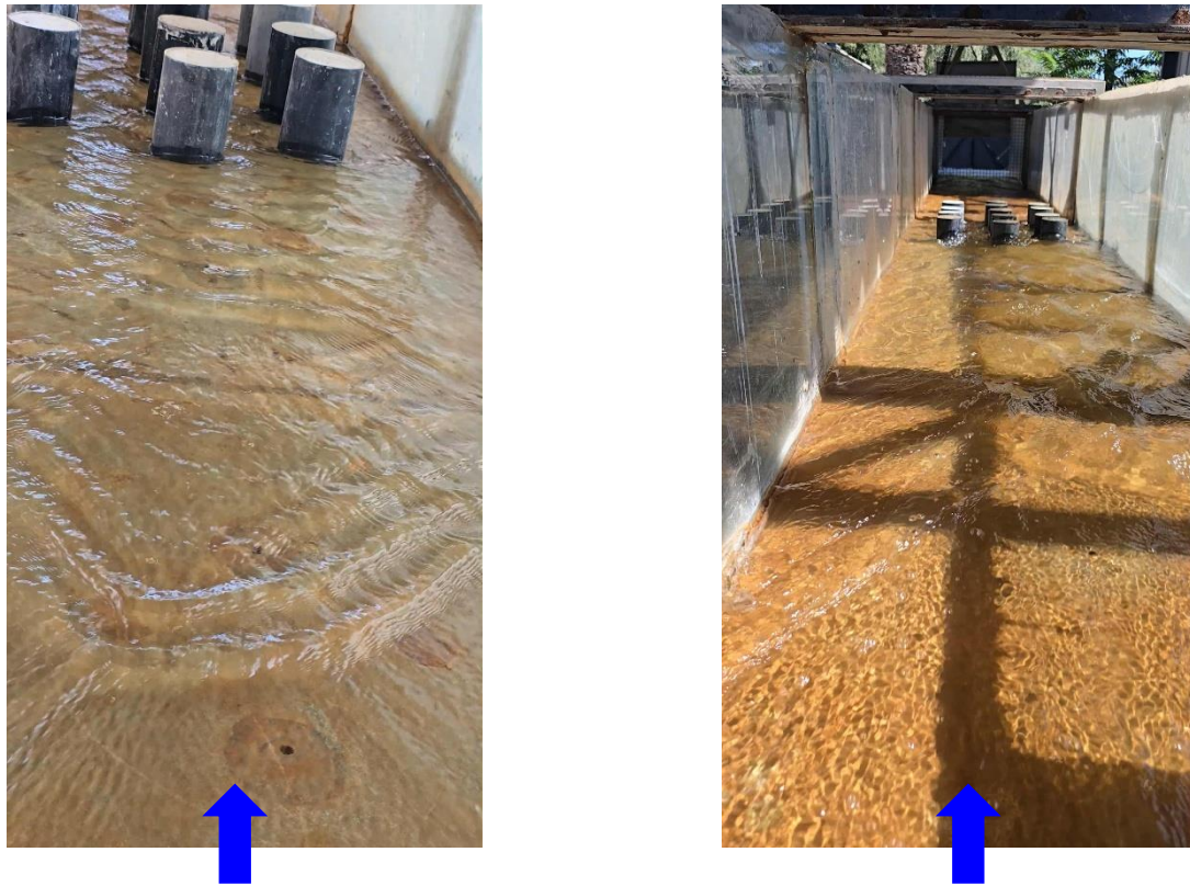
Figure 7. Evolution of Turbulent Zone Length ( L_{\text{turbulence}} ) and Mean Water Height ( H_{\text{mean}} ) Upstream of Obstacles for the Obstacle Configuration across Increasing Discharges
