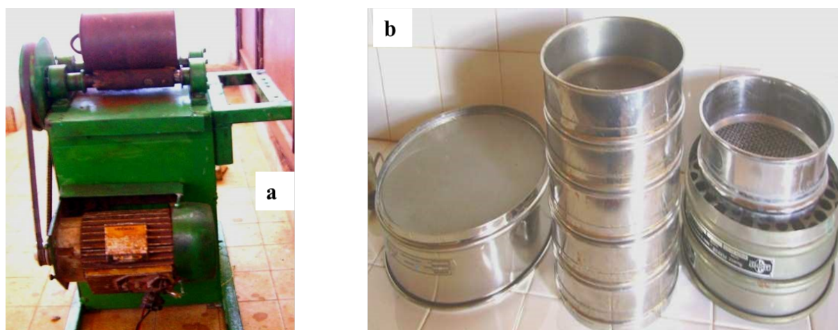
Figure 2. a: The ball mill. b: Sieves with different mesh sizes (500, 250 et 80 µm).
